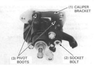
Position the caliper with the piston down and apply small squirts of air pressure to the fluid inlet to remove the piston.
