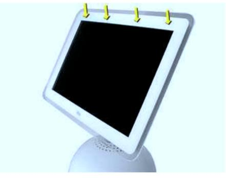
2. Holding onto the display, turn it over and lay the display face down on a soft cloth. Push the rear housing in the direction of the arrows. This will mate the housing and display tabs.
