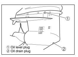
4. Fill with recommended gear oil through oil drain hole until oil just starts to flow out from oil level hole.
